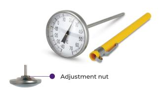
These pocket-sized  $\emptyset$ 45 mm dial thermometers feature a pointed  $\emptyset$ 4 x 130 mm stainless steel stem. Each dial is manufactured in three scales and is supplied with a FREE calibration spanner and probe cover complete with pocket clip.
