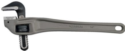
Handle made of extremely lightweight aluminium which is as robust as heavy-duty cast iron. Jaw opening sits parallel to the handle making it ideal for overhead applications. Narrow jaw head makes it easier to use within tight areas. Pipe capacity 60mm/2 3/8". Length: 350mm/14".
