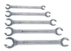
Conform to ASME B107.4. Made from high quality chrome vanadium steel. Satin finish body with highly polished heads. Offset ends. The wrench will fit over the pipe to give a positive location on the nut. Can be used on hydraulic pipes, brake pipes etc. Contents 1/4" x 5/16", 3/8" x 7/16", 1/2" x 9/16", 5/8" x 11/16" and 3/4" x 7/8".
